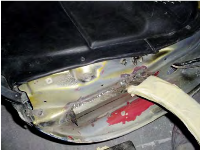
11. Grind, scuff the welds surface & mask undercoat paint & top coating to prevent rust.
