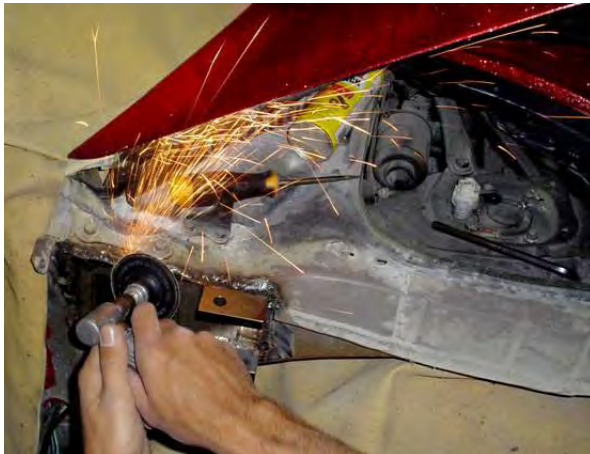
11. Grind, scuff the welds surface & mask undercoat paint & top coating to prevent rust.
